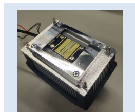
Chip-on-Board LEDs (24 W optical power/unit)
